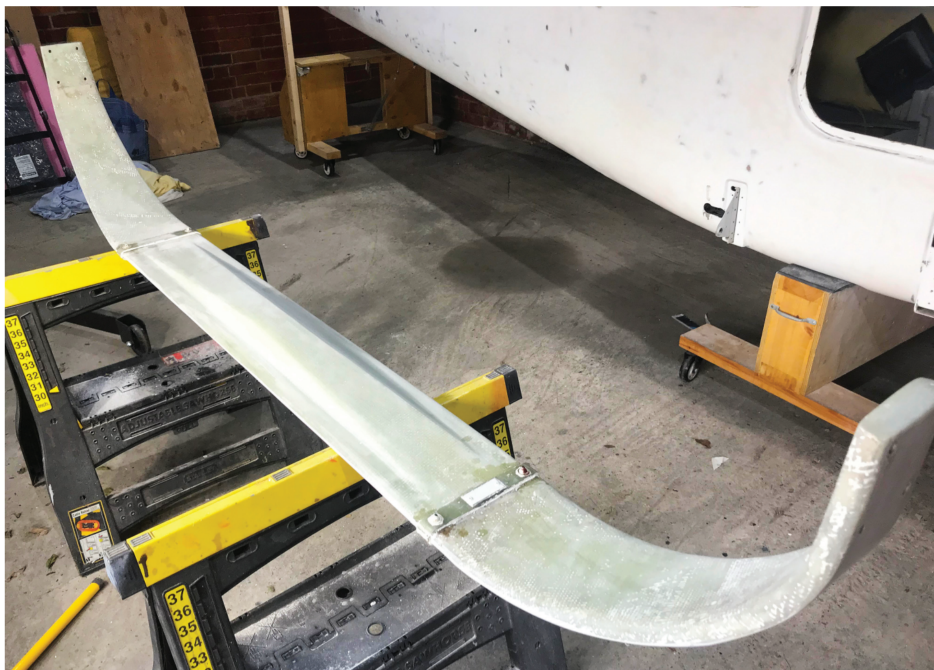
Above The GRP undercarriage 'spring' stripped of paint for inspection. Photo: Berian Griffiths
